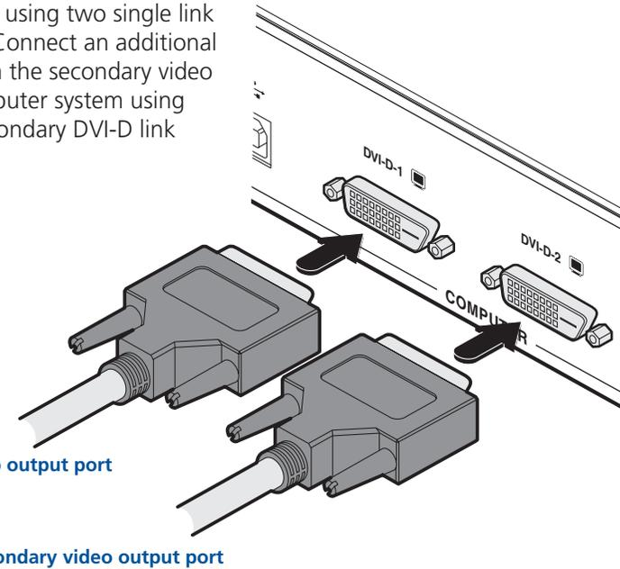
[ALIF2000 when using one very high resolution DVI-D dual link display] Use a DVI-D Dual Link cable (such as Adder part: VSCD3) to connect the primary video port of the computer system to the DVI-D-1 connector of the ALIF2000. A dual link cable must also be used at the RX unit.
