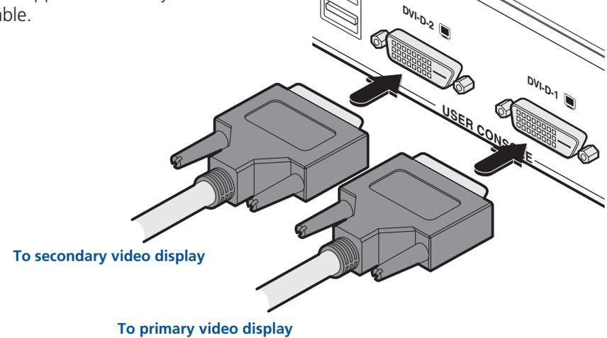
[ALIF2000 when using one very high resolution DVI-D dual link display] Use a DVI-D Dual Link cable (such as Adder part: VSCD3) to connect the video display to the DVI-D-1 connector of the ALIF2000 RX unit. A dual link cable must also be used at the TX unit.
