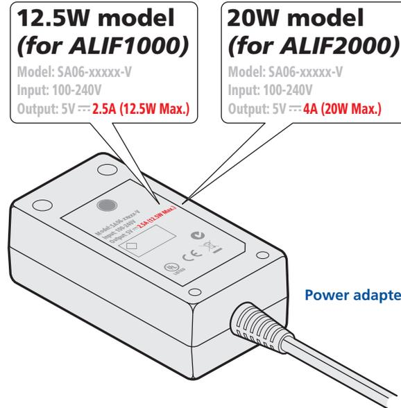
No damage will be caused if the 12.5W adapter and the 20W adapter are used in place of each other on either of the ALIF1000 or ALIF2000 units. However, correct operation of ALIF2000 units can only be guaranteed if a 20W power adapter is used. Always ensure that only ADDER 5-volt power supplies are used to power the units.
