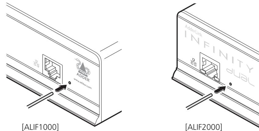
**Use a straightened-out paper clip to press the reset button while powering on the unit**
