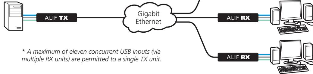
*\* A maximum of eleven concurrent USB inputs (via multiple RX units) are permitted to a single TX unit.*
